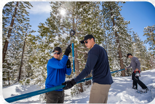
Manual snow survey, measuring the depth and weight of snow.
