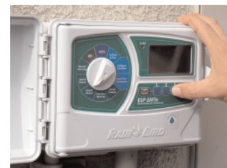
Smart controllers use weather data to automatically set irrigation cycles.
